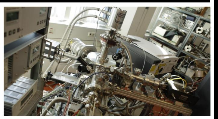
$p \sim 10^{-10} \text{ [mbar]}, T = 15 \text{ [K]}$ H flux: 8x10<sup>12</sup> [cm<sup>-2</sup> s<sup>-1</sup>] Molecular fluxes: 3x10<sup>11</sup> [cm<sup>-2</sup> s<sup>-1</sup>] Ice thicknesses: 10-20 monolayers
