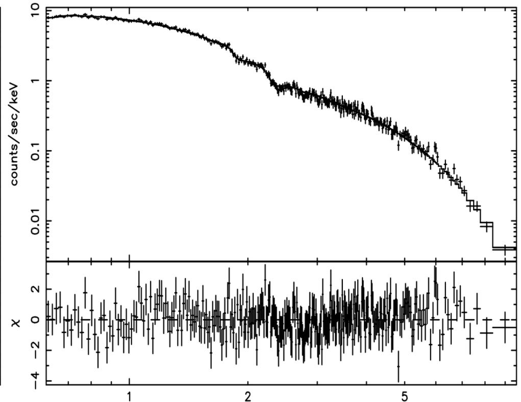
Synchrotron spectrum:  $S(E) = K E^{-a-b \log(E)}$   $b \approx \frac{r}{5}$
